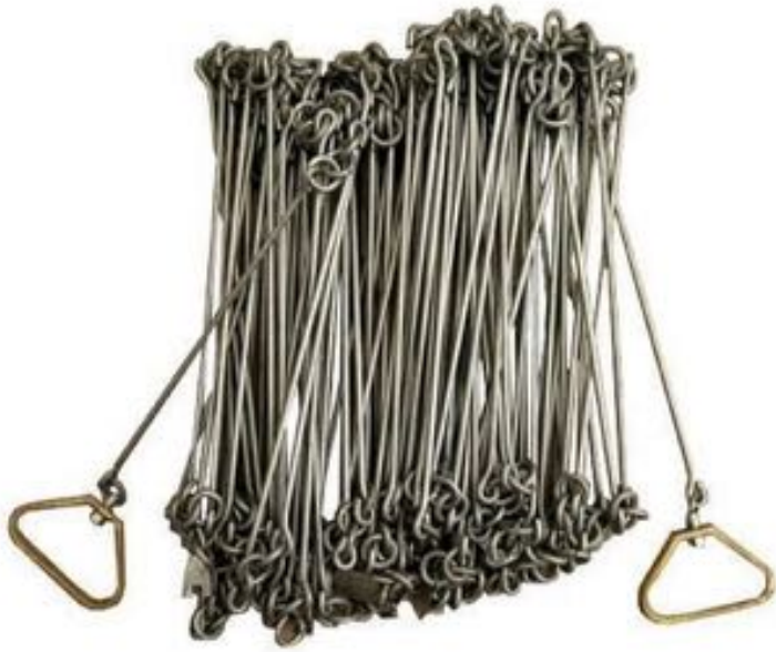
Gunther's chain for distance measurement in chains and links, 22 yds in length, 100 links per chain.
